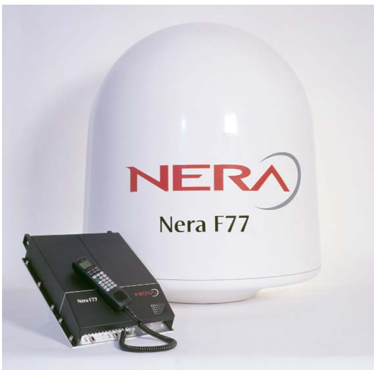
Figure 5 Ship earth station Nera F77, which belongs to the so-called Fleet range of services; capacity 64 kbit/s for voice and data – global coverage. World market share 41 per cent
