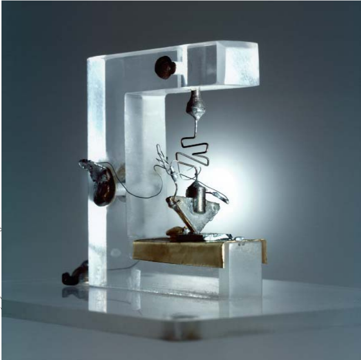
In 1950, an article from a study tour to USA the year before presents both mobile telephony and the newly invented transistor. The transistor invented by Bardeen, Brattain and Schockley in 1947 was of the point-contact type. The original is on display at Bell Labs lobby exhibit, open to the public, at Lucent Technologies headquarters in Murray Hill, NJ, USA
