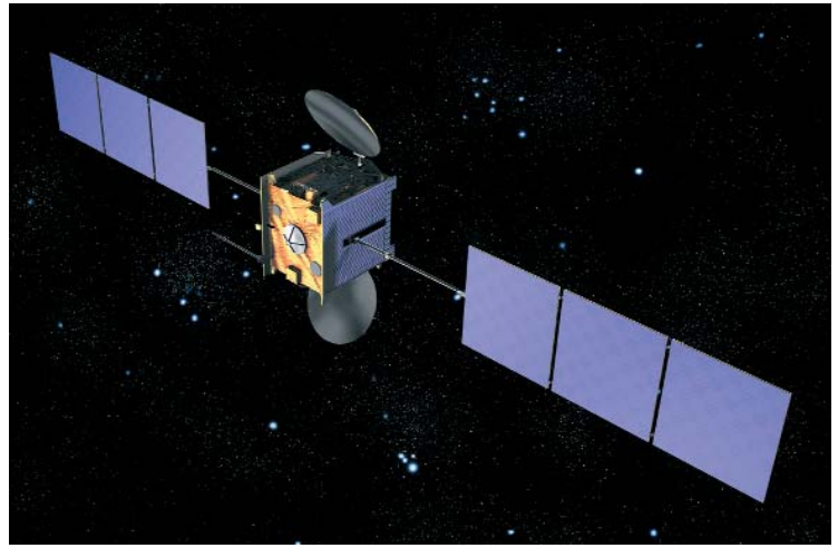
Figure 4 The third generation INMARSAT satellite. Essential new feature: seven spot beams (five active) in addition to global coverage. The spot beams gave extra capacity in areas where demand from users was high, and furthermore allowed the introduction of the mini-M standard mobile station – see Figure 6
