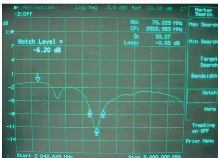
Figure 9 Reflected power for a 5 patch array
