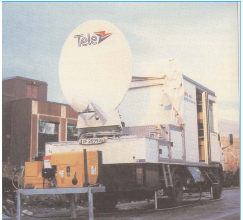
Figure 2 1.8 m antenna on transportable earth station
